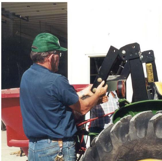
Fig. 1. Manually adjusted ROPS down.
