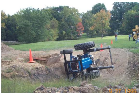
Fig. 6. As the tractor rolls over the AutoROPS deploys (raises).
