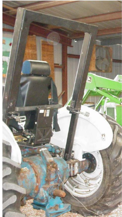
Fig. 4. AutoROPS deployed.
