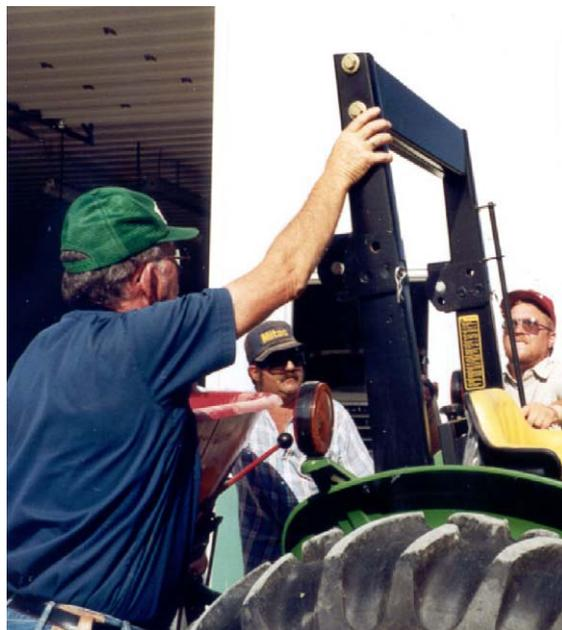
Fig. 2. Manually adjusted ROPS up.
