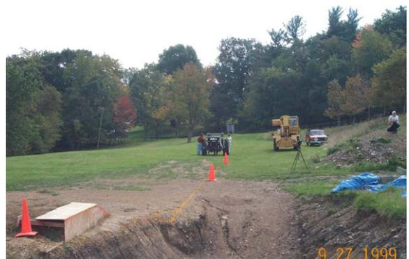
Fig. 5. Tractor approaching rollover pit with AutoROPS in low-profile position.
